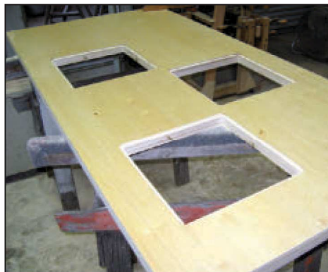
■ FIGURE 8. Window holes cut and routed in the kiosk panels.
