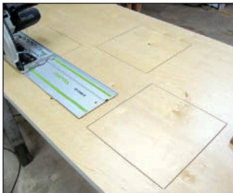
■ FIGURE 7. Cutting the window holes in the kiosk panels.
