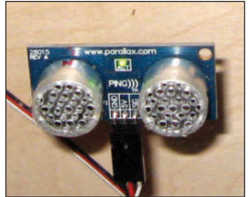
■ FIGURE 17. The Parallax Sonar Sensor mounted behind the plastic window.
