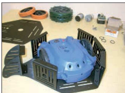
■ FIGURE 2B. A Parallax Scribbler robot easily fits inside the Stingray's roomy chassis.
