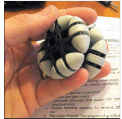
■ FIGURE 11. The multi-directional tail wheel can roll in any direction.
