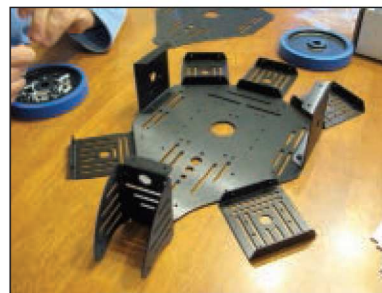
■ FIGURE 6. The main chassis parts laid out and ready to assemble.
