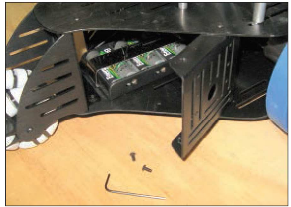
■ FIGURE 12. With two screws removed, a battery access door is created.
