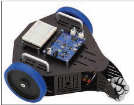
■ FIGURE 9. The mounted MSR1 board and adjacent breadboard ready for experimentation.
